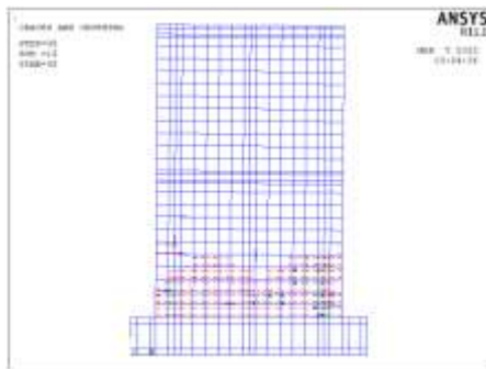
Fig 15.a. Cracking pattern at failure load (front/back elevation) –Model (S-01-FEM-M).
