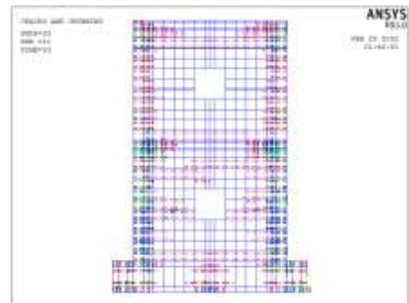
Fig. 8.f. Cracking pattern at cracking load (at ultimate load) for face with windows.
