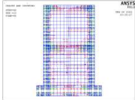
Fig 10.g. Cracking pattern at cracking load (at failure load) for solid face - model (S-02-FEM)
